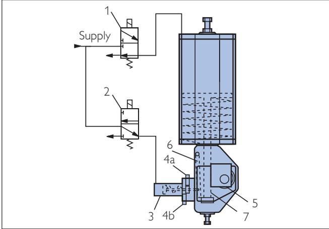
Figure 1. Automated jammer, "spring-to-close" actuator
