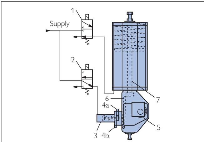
Figure 2. Automated jammer, "spring-to-open" actuator
